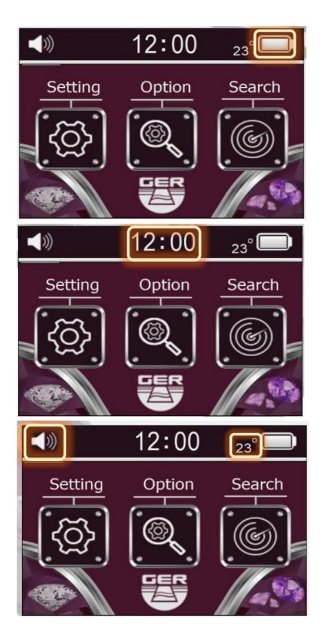
After turning on the device, the following data will appear on the main screen: Battery level indicator – clock – temperature – activate and mute button.
