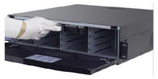
5. Buckle up the hard drive and close the front panel
