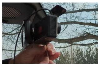
6. Route the cable between the headliner and roof towards the A pillar. Remove the door gasket and cover on the A pillar so that you can route the cables underneath the curtain airbag.
