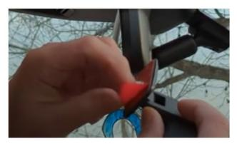
5. Slide the sensor unit into the bracket and use the provided locking tool to tighten the unit in place, ensuring the sensor is facing level and forward.
