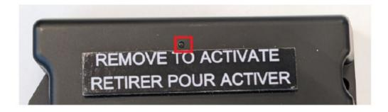
\* NOTE: Place the magnetic strip approximately 13 to 14 mm from the bottom edge of the device. For additional information, see FAQ here.
