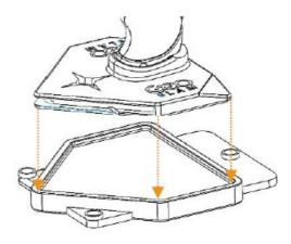
• At the end of each scan, return the scanner to the initialization base before powering off the scanner.
