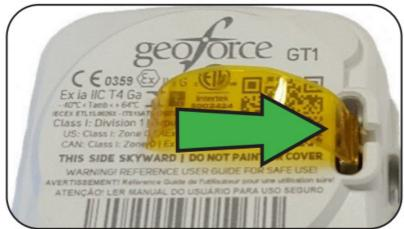
This magnet insertion aborts any ongoing radio message event and prevents any new radio message events from starting. This is equivalent to the OFF state.
