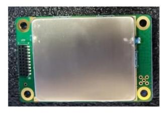
Note: 20PIN-connect to host, input and output data
