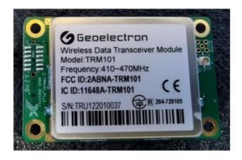
Note: IPX port connect antenna, radio frequency signals are received and transmitted
