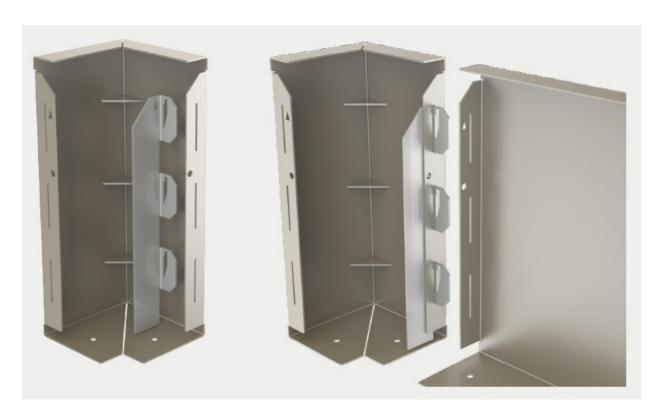
**Step 03**Slide the locking key onto the exposed lugs, push forward and down to engage the locking teeth. Now start the process again with the next sections.
