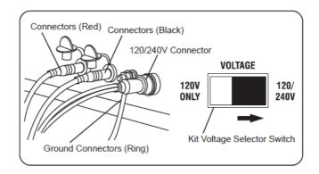
**Note**: The grounding end of the kit should be connected to the ground screw and grounded.
