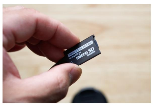
4. Open the M2 slot cover on the PSP Go and Insert the adapter in. Once you slot it in, you should hear a clicking sound which means the adapter is inserted and the system should be reading it. If you don't hear a clicking sound, make sure you're pushing it in until it clicks.
