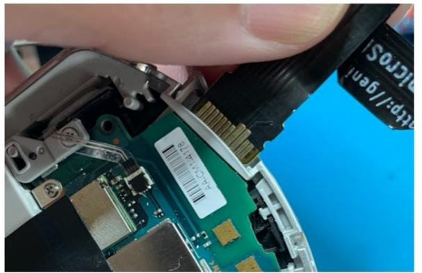
5. The adapter cable should easily slot into the back of your PSP Go, so now just place a piece of heat-resistant tape or black tape (either is recommended) to hold the Memory Stick PRO Duo card and another piece to hold down the right and left side of the adapter cable as shown.
