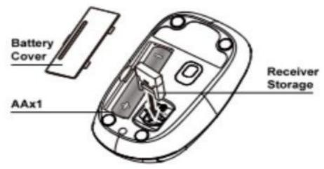
Remove the battery cover from the keyboard.Install one AA batteries Into the keyboard.
