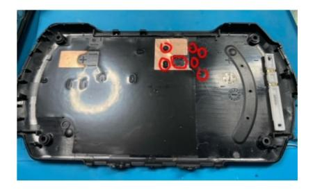
Additionally, you will want to cut flush the small plastics in the highlighted area below. This will help reduce any bulging caused by the SD memory card reader.
