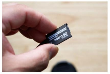
4. Open the M2 slot cover on the PSP Go and Insert the adapter in. Once you slot it in, you should hear a clicking sound which means the adapter is inserted and the system should be reading it. If you don't hear a clicking sound, make sure you're pushing it in all the way until it clicks
