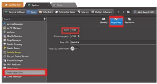
Click [Properties] in [Web-based SDK]. Confirm the Port Number. The Default Port number is 4590. (This port number is used in Step 3.1.)
