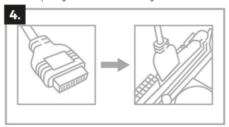
5. Connect the case fan distributor to the FAN connector on the motherboard. The speed of the fans can be controlled from the motherboard's UEFI or the included Windows application.
