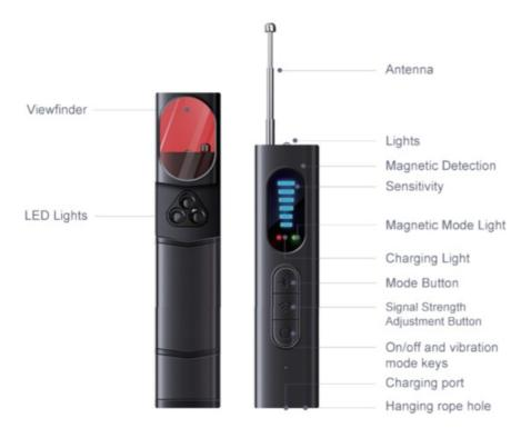
A:Detection of radio waves (wireless cameras/eavesdroppers, etc.)
