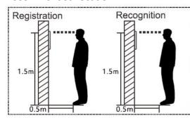
When using the device for registration and identification, the installation location of the device must remain unchanged. If you really need to move the device, you must keep the installation height consistent. If it is inconsistent, it may affect the recognition effect. It is recommended that the distance between the face and the machine at the time of registration is 0.5-0.8 meters.
