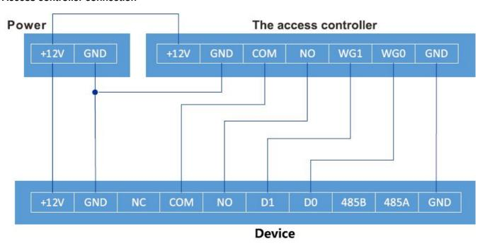
**Note:** The combination of NO and COM is normally open, and the combination of NC and COM is normally closed, respectively to the NO, NC and COM terminals of the access controller. The corresponding wiring mark is printed on the 10PIN interface, please refer to the actual product
