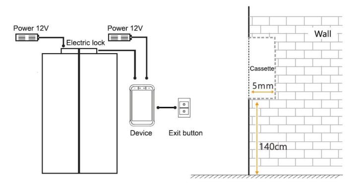
sets of wires need to be embedded in advance at the host equipment (reserved wire length is 10cm):
