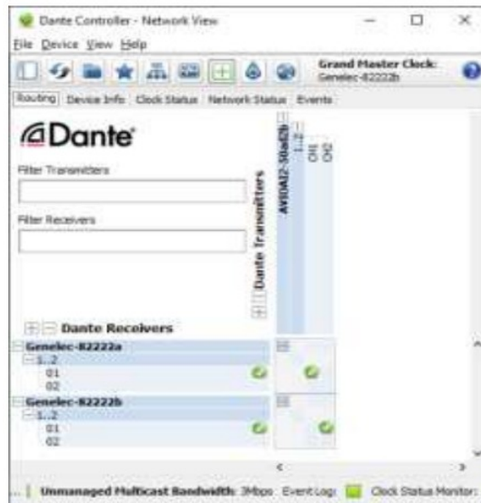
Figure 7. Configuring for AES67/ST2110 streams in the Dante controller.
