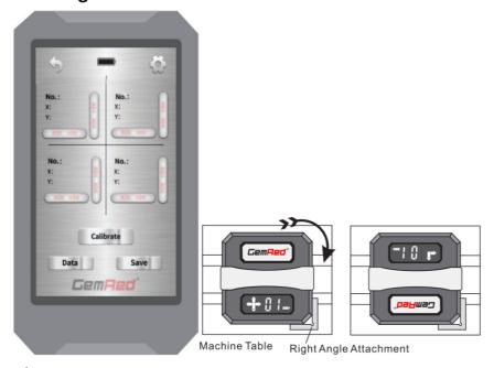
Note: When calibrating, please keep the measuring surface of the levelling device and the table surface in full contact, rotate the angle to 180° as far as possible, the table surface is flat, no vibration, no impurities or grease accumulation, it is recommended that
