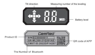
**Tilt direction:** The arrow pointing or the increasing direction of the square is the direction of high inclination of the measured surface, which can guide the rough adjustment of the level of the surface.
