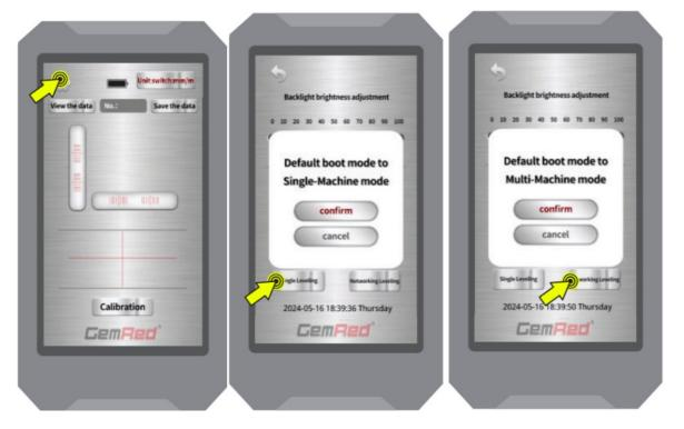
When use the handheld terminal for the first time, it defaults to stand-alone mode (single leveling) Ignore this step if you do not need to switch.
