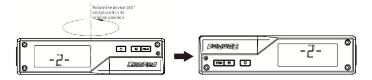
**Step 3**: Short press the button, the display will flash and display "-2-". Keep the device stationary until the display flashes and displays "CH 1", indicating that the second step of calibration is completed. At this time, it enter the calibration self check mode. Keep the device stationary until the LCD displays "CH2"
