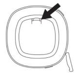
Open the battery cover. Insert the battery and make sure the positive pole face up.
