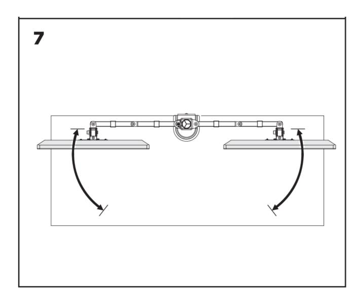
**Note:** if the display does not stop at your desired position , tighten the screws as shown.
