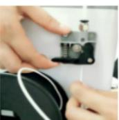
Press the Knob to start loading filament. Once filament starts extruding from the Nozzle, press the Knob again to stop extrusion, then press the Knob to select the Continue option.
