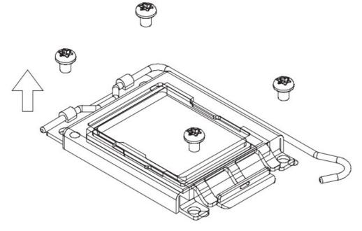
2. Remove the original LGA1700 CPU mounting.
