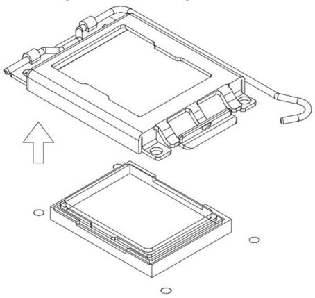
3. Apply the CPU Protector Frame on top of CPU and tighen the screws.
