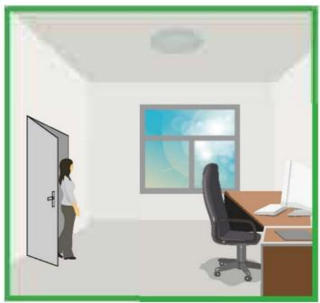
With suffcient naturallight, the light does not switch on when presence detected.
