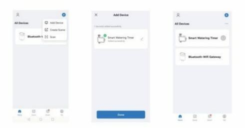
Step ②.Once the connection is completed, the paired device will be listed on the home screen. Tap the "Bluetooth-Wi-Fi gateway" icon to enter the device details screen.
