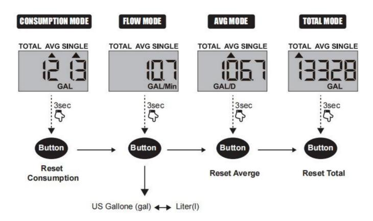
Press the button directly, the display switches to next display mode.
