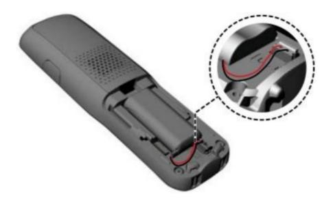
Align the cover flat against the battery compartment, and then slide it upwards until it clicks into place.
