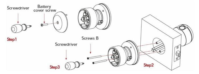
Note: The UP↑ faces upwards. After adjusting the Interior Knob, tighten the screw B.
