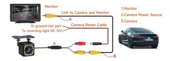
Please connect A/B to the video input trigger wire, ONLY WHEN some monitors may require additional trigger signals to display the reversing image. (This model does not require this connection)
