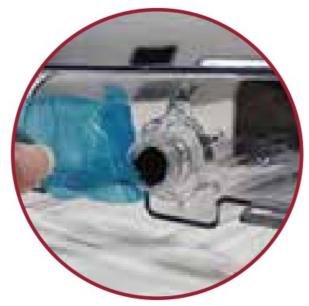
2. Before making espresso, make sure the knob is on the  $\mbox{OFF}$  position.
