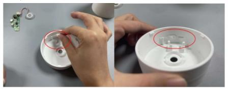
5. Place the ⑤ main board into the ① upper cover, align it with the positioning pillar, press it firmly, and place the atomizer with the front side facing up (as shown below)
