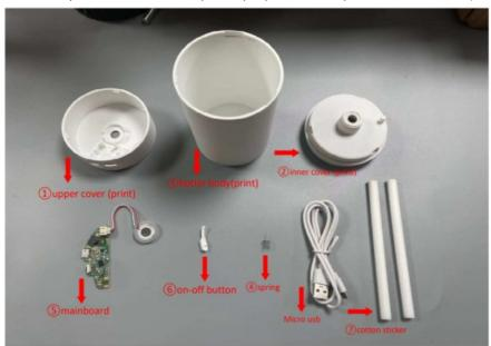
4. Place the ⑥ on-off button into the ① upper cover, making sure to place it behind the positioning pillar (as shown below)
