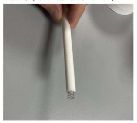
8. Insert the cotton sticker with the spring installed into the bottle (as shown below)
