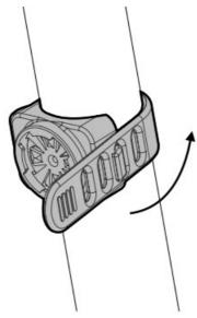
3. Insert the holes on the silicone tape into the base slot and bend the remaining silicone tape backwards;
