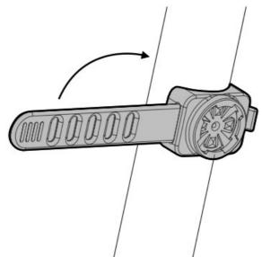
2. Place the base on the seat tube and wrap the silicone tape around the handlebar;
