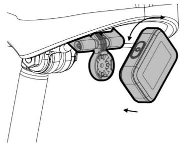
3. Align the protrusion at the bottom of the lamp holder with the notch on the lamp holder, press it into the bottom, and rotate it 45 degrees;
