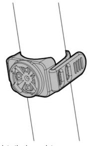
4. Insert the other hole on the silicone tape into the base slot;
