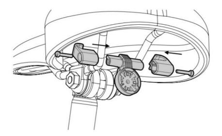
1. Secure the left and right fasteners of the lamp holder onto the base bow and insert the left and right screws;
