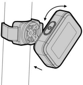
5. Align the protrusion at the bottom of the lamp head with the notch on the base, press it into the bottom, and rotate it 45 degrees;
