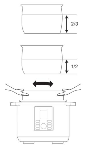
Overfilling may clog the pressure limit valve, which can cause excess pressure to develop. Always use at least 1/2 cup liquid when pressure cooking.
