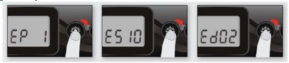
This mode allows you to lower the temperature set point of the spa by  $20 \, ^{\circ}F(11 \, ^{\circ}C)$  during a certain period of the day. The display will show EPx, "x" representing the state of the programmed economy(0 = disabled, 1 = enabled). Use the arrow keys to enable or disable economy mode. Use the Light key to jump to the next parameter, economy start time (ES).
