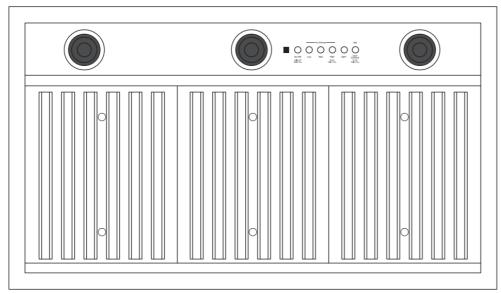
Adjustable CFM blower – High-powered 610-CFM blower range hood, adjustable downward to either 370 or 290 maximum CFM to accommodate different installation needs
