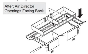
5. Replace blower plate with the screw removed in Step 1. Make sure the screw is tight.
