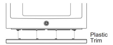
• Installation Above 36, align trim tabs on the plastic or metal trim to slots in the bottom of the oven.
