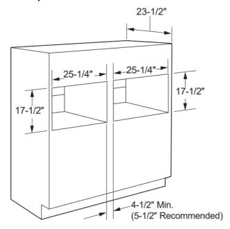
• If you are mounting a Speed Cook Oven beside another, use the dimensions shown. The middle rail separating the two openings may need to be larger than the 4-1/2 minimum shown.
