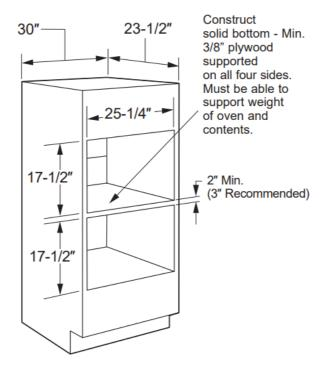
• The support must be level and rigidly mounted, flush with the bottom edge of the cutout.
