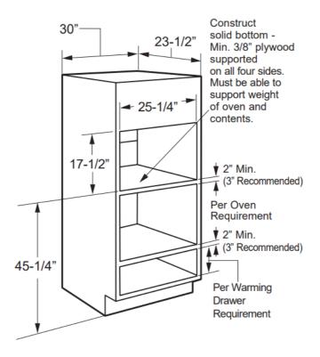
**NOTE:** Additional clearances between the cutouts may be required. Check to be sure the oven supports above the Warming Drawer location does not obstruct the required interior depth and height. See Warming Drawer installation instructions for details.
