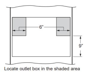
Install a recessed electrical outlet in the back wall of the opening within 6" of either side and at least 9" above the cutout floor.
