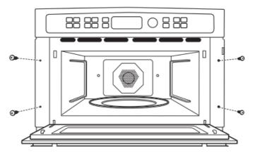
• Slide the oven the remaining way into the opening so that the side flanges and control panel are against the
