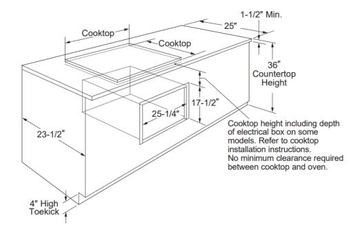
Gas or electric cooktops may be installed over this oven. See cooktop installation instructions for the cutout size. See the label on top of the oven for approved cooktop models. This oven requires a separate, properly grounded 15-Amp, 120-Volt, 60Hz power supply. The cooktop requires a separate power supply. Use a 30 or wider base cabinet.
