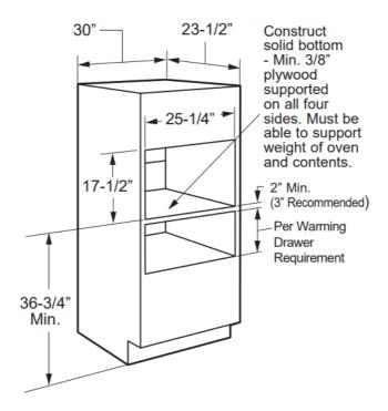
**NOTE:** Additional clearances between the cutouts may be required. Check to be sure the oven supports above the Warming Drawer location does not obstruct the required interior depth and height. See Warming Drawer installation instructions for details.
