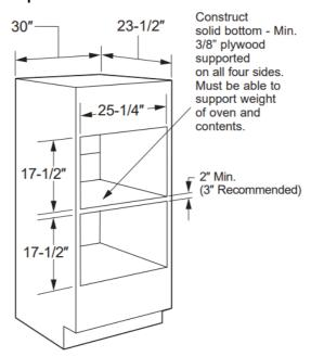
• If you are mounting a Built-In SpeedCook Oven over another, use the dimensions shown. The middle rail separating the two openings may need to be larger than the 2 minimum shown.
