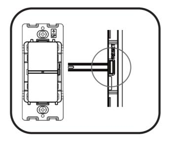
To reset the network of the device, remove the faceplate from the device. Then press and hold the reset button for 5 seconds. Install the faceplate back onto the device.
