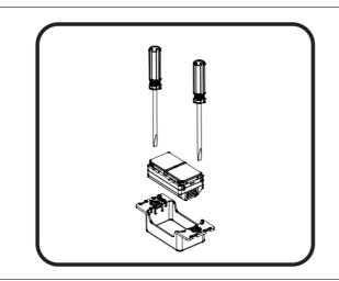
Use a standard screwdriver to remove the devices f rom the back housing
