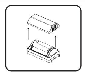
Separate the battery cover from the device. Pull the plastic in rip out of the battery compartment.
