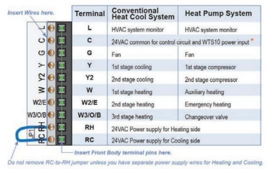
\* A common connection between the HVAC unit and the "C" terminal is required.
