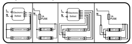
8. Install the retrofit kit Caution label in an easy to see location to ensure the user understands the system now uses LED Type B double ended tubes, and the use of fluorescent lamps may result in damage or injury.
