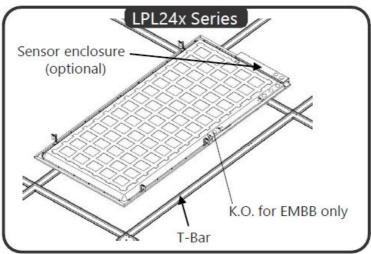
4. Bend the brackets on the housing to make sure they hook to T-Bar.
