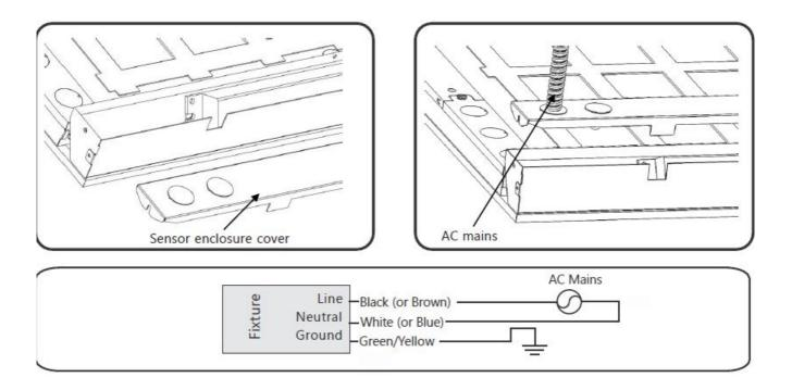
1. Remove sensor enclosure cover. Carefully remove knockout for ACmains input wires. Install UL listed electrical fittings in the knockout holes for wire protection.
