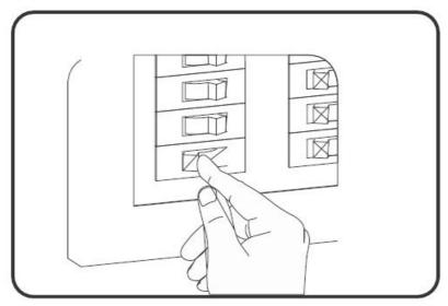
2. Default lumen level is M(medium), and default CCT is 4000K. For other lumen level or CCT, loosen screw and remove switch cover, then set switch to the desired lumen level or CCT by screwdriver. Re-attach cover and tighten screw.
