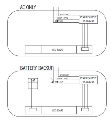
**NOTE:** Connect to a single source of power supply so that all lamps are simultaneously illuminated.
