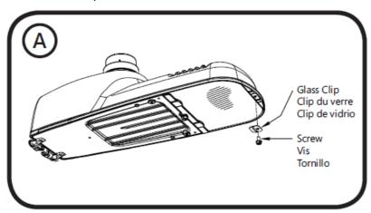
2. Slide on Refractor Over Rim of Luminaire
