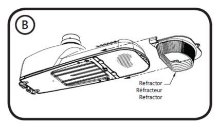
3. Secure with Front Lens Screw & Glass Clip.
