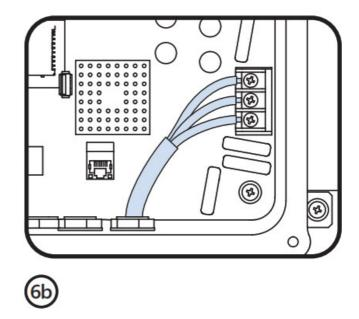
Insert the power feed cable throu gh the cable gland in the bottom o f the Gateway enclosure. Strip each wire no more than 0.25". Route the power cable as tightly as possible (avoid larger than necessary loops/slack) to the terminal block inside the enclosure. Avoid touching any other component on the Gateway circuit board.
