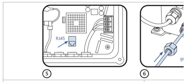
Push the cable through the sealing gland, and plug it into the RJ45 Ethernet jack on the circuit board.
