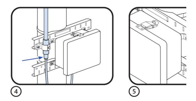
Connect the Coax RF Cable to the RF Antenna: The RF Cable is pre-installed on the gateway assembly. At tach to the screw terminal on the bottom of the RF Antenna, and tighten securely.
