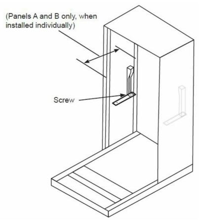
• STEP 6: If installing a 2-piece baffle configuration(for deeper plenums only) that requires 2 baffle plates to be used in tandem, install the front 2 baffle extension legs: (When installing A+C or B+C baffle plates)
