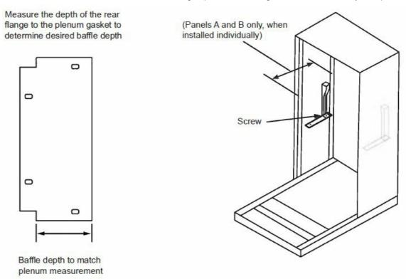
• STEP 7: Install the previously selected baffle plate and secure it with either 4 or 6 screws (depending on the depth of the baffle plate selected):
