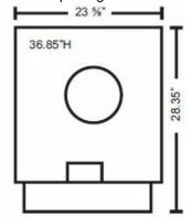
NOTE: For side installation configuration a service opening of 31" is recommended
