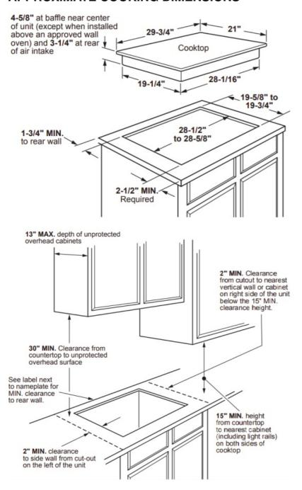
To insure accuracy, it is best to make a template when cutting the opening in the counter
