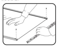
4. Remove the old diffuser by sliding it toward the side without end rail. Insert new diffuser, keeping the round corner of diffuser on bottom left.
