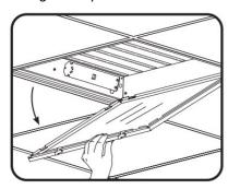
3. Place front bezel with diffuser on table. Unfasten the two rail screws on the end rail with latches, then remove this end rail.
