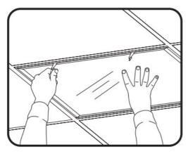
2. Swing down panel and lift off front bezel with diffuser.
