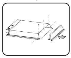
7. Install the fixture back to the ceiling. Connect the AC and dimming wires.
