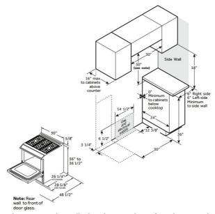
**Note:** Minimum to bare cabinet above; see Installation Instructions for alternate installation configurations.
