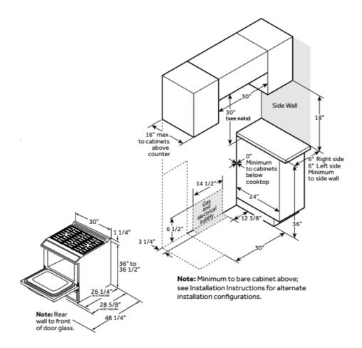
**Note:** Cabinets installed adjacent to slide-in ranges must have an adhesion spec of at least 194° F (90° C) temperature rating.
