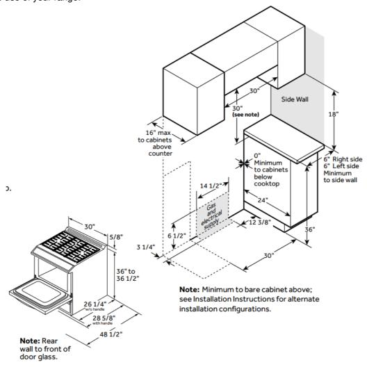
Allow 30" (76.2 cm) minimum clearance between burners and bottom of unprotected wood or metal cabinet, or allow a 24" (61 cm) minimum when bottom of wood or metal cabinet is protected by no less than 1/4" (6.4 mm) thick flame-retardant millboard covered with no less than No. 28 MSG sheet metal (.015" [.38 mm] thick), .015"
